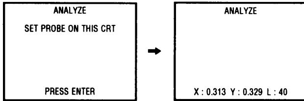
If the above screen is not displayed after 30 seconds or more, disconnect the connector from the OPTION terminal and connect it again, then press the ENTER button. If the symptom does not change, the monitor is defective.
