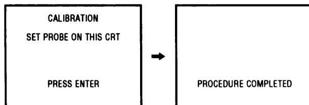
3-11. Set the color temperature of the monitor to COL1, then set the luminance to 40cd/m<sup>2</sup> adjusting the contrast control and record the x and y values of the color analyzer.
