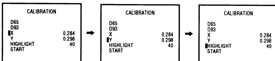
3-16. Attach the BKM-14L to the CRT and press the ENTER button.
