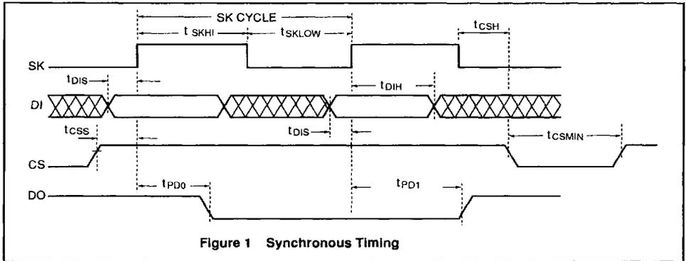
Figure 1 Synchronous Timing
