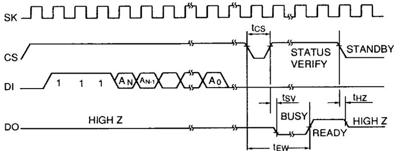
After an ERASE instruction is shifted in, CS is dropped low. This sets the beginning of the self timed erase sequence. If CS is then brought high (after observing the  $t_{cs}$  spec) the DO pin will act as a status indicator. It will remain low so long as the chip is programming. It will go high after all the the bits of the addressed register are set to a logical 1.
