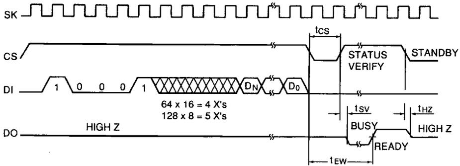
The WRAL instruction writes to all the registers simultaneously. All the registers must be erased before a WRAL operation. Except for its different opcode, the WRAL instruction is identical to the WRITE instruction.
