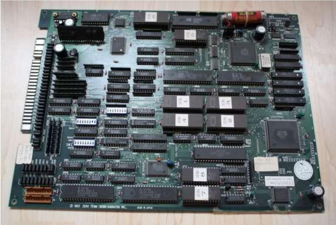
Some PCBs use an extra PLD (PAL or GAL) mounted on a PLD which can be removed for the battery-less program.
